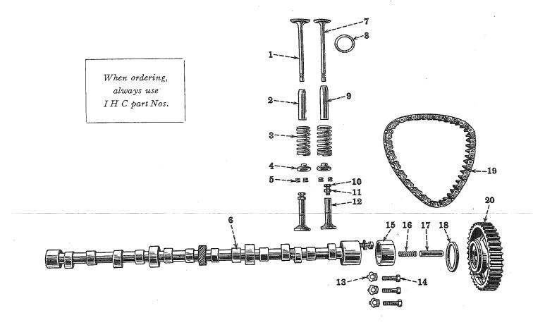
Valves, Guides, Springs, Tappets, Camshaft, Bushings, Sprocket, Chain
