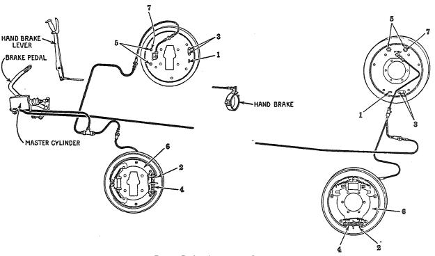
Fig. 1, Brake Adjustment Diagram
