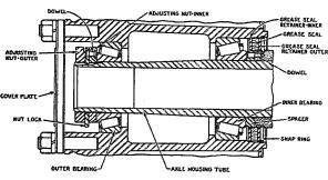
Fig. 15, D-246T Rear, Trailing
