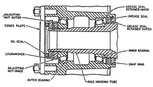
Fig. 13, D-186T, DS-186T Rear, Trailing
