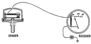
Fig. 3, Oil Pressure Gauge-No Pressure
