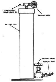
Fig. 28, Test Tank
