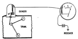
Fig. 2, Gas Gauge-Tank Full
