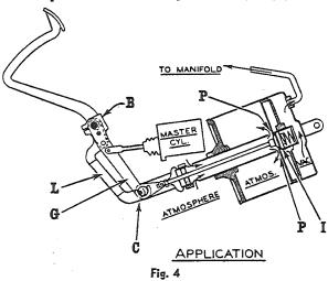
The valve is now moved to the closed or applied position as shown in Fig. 4. Atmospheric pressure is admitted, through the air cleaner, the connecting tube, the end plate cover, the hollow piston rod, and ports (P) of the valve to the space forward of the piston, partially destroying the vacuum; vacuum is still maintained on the opposite side of the piston. The piston now moves forward due to the difference of pressure.
