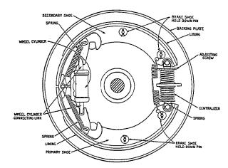
Fig. 3, Front Brake
