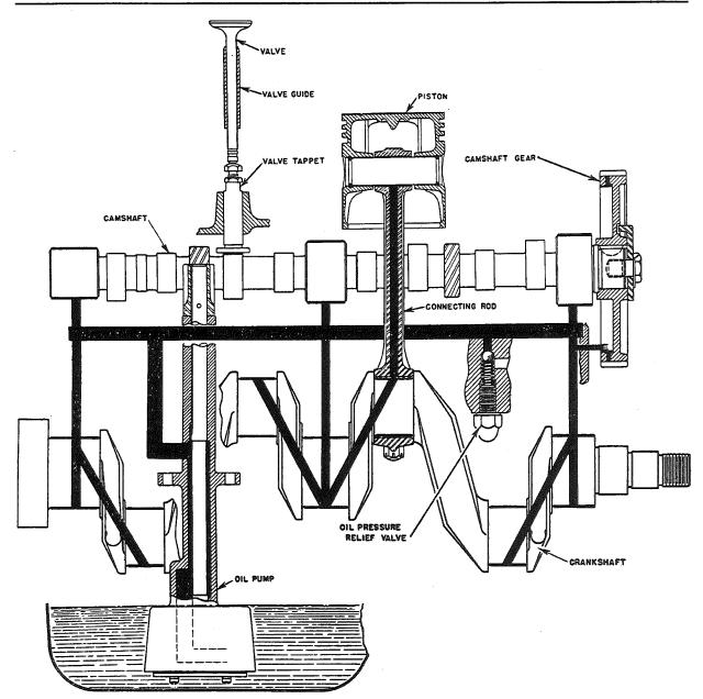
Fig. 17, Engine Lubrication System
