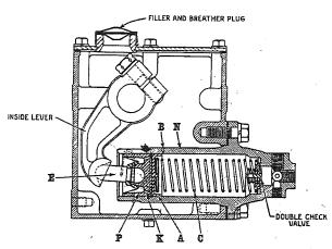
Fig. 2, Typical Box Type Master Cylinder
