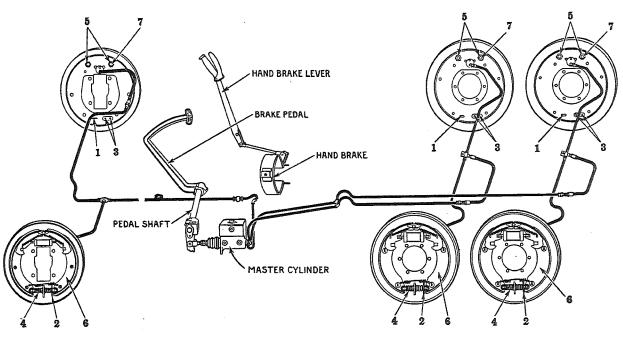
Fig. 1, Brake Adjustment Diagram
