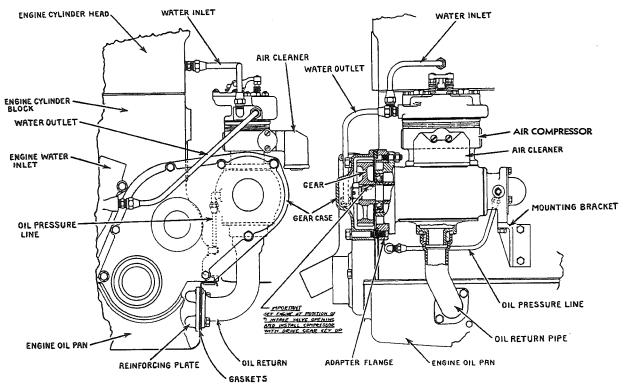
Fig. 8, Air Compressor Installation
