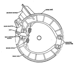
Fig. 2, Front Brake
