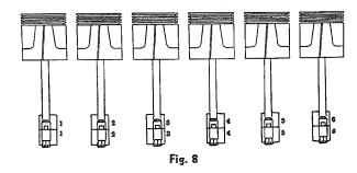
Connecting-rod bearings are installed flush with face of connecting rod and cap at tongue and groove side, which permits the lower half bearing to extend above face of bearing cap on opposite side.
