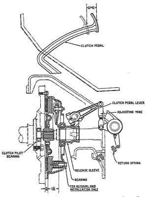
Fig. 7, Clutch Control (D-35, D-35B, DS-35, D-40, D-216T)
