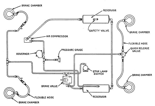
Fig. 1, Typical Air Brake Installation (4-Wheel)
