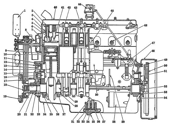
Fig. 3, FBB-361, FBB-401, FBB-450A Engine
