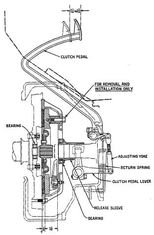
Fig. 8, Clutch Control (D-50, D-60, DR-60, D-246T, D-246F)
