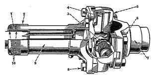
Fig. 2, 10 Splines on Propeller Shaft
