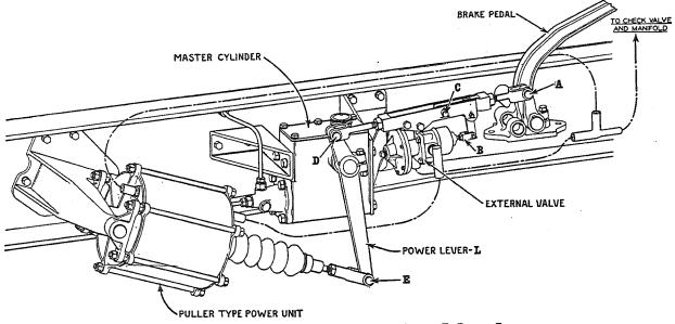
Fig. 7, Vacuum Power Unit Installation—D-246T, D-246F (See Page 1 for Other Models)
