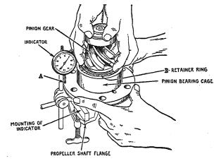
Fig. 2, Checking End Play of Pinion Bearing
