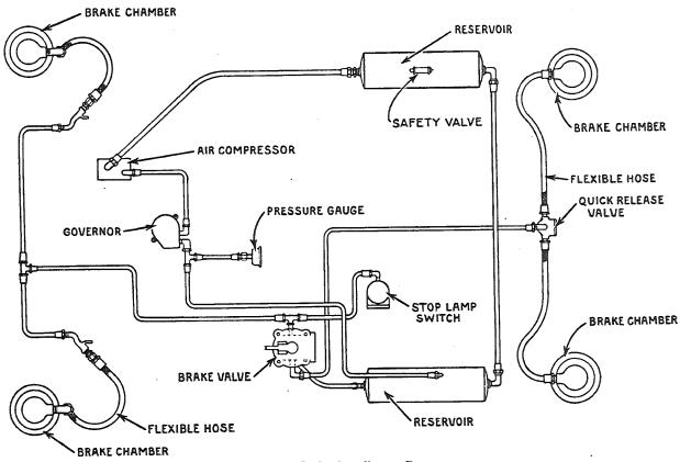
Fig. 1, Air Brake Installation Diagram
