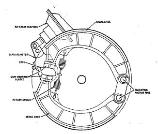
Fig. 2, Front Brake
