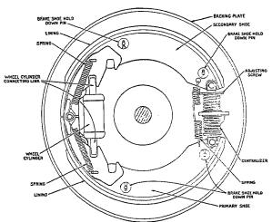
Fig. 4, Front Brake
