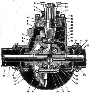
Fig. 2, R-1300, R-1400, RB-1400, RT-1400, RF-1401 Axle
