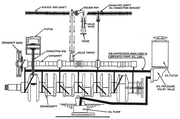
Fig. 38, Engine Lubrication System
