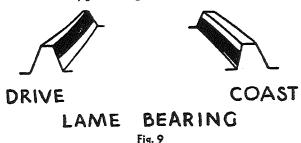
Fig. 9 shows a lame bearing; gears can be adjusted to obtain a good driving condition but poor coast or reverse.
