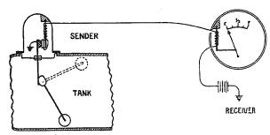
Fig. 1, Gas Gauge-Tank Empty
