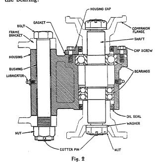
When assembling the bearing in the housing it may be necessary to tap the outer race slightly to start it in the housing bore. After the bearing race is installed, a slight pressure should move it freely. If any binding is felt, scrape or lap the housing bore to obtain the proper fit.
