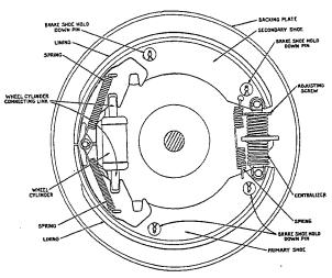
Fig. 3, Front Brake
