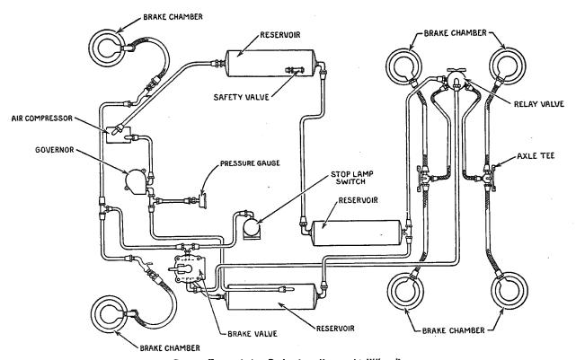
Fig. 2, Typical Air Brake Installation (6-Wheel)
