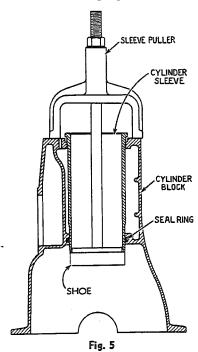
When replacing cylinder sleeve be sure there is no dirt under sleeve flange which would cause distortion. Before installing rubber seal ring, see that sleeve revolves freely in cylinder block bore.
