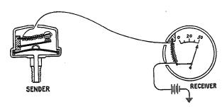
Fig. 4, Oil Pressure Gauge-With Pressure
