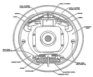
Fig. 3, Front Brake
