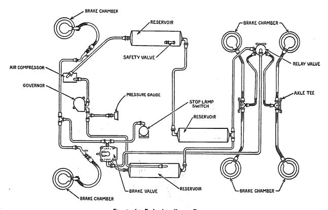
Fig. 1, Air Brake Installation Diagram
