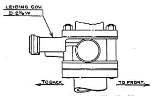
Fig. 1, Governor Installation (B-21/2-W and B-3-W)
