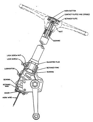
Fig. 1, RT-260 Steering Gear
