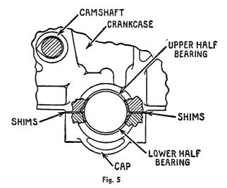
IMPORTANT: Before installing new bearings be sure to clean out drilled oil passages in crankshaft and block. A rifle barrel brush or a brass rod should be run thru the oil passages to dislodge any sludge, grit or bearing material. Plugged oil passages will prevent adequate lubrication to the new bearings, resulting in early failure.
