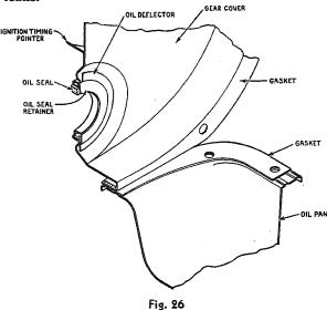
Fig. 26 illustrates the assembly of the crankshaft front seal, retainers and oil pan gaskets and Fig. 27 illustrates the rear assembly.
