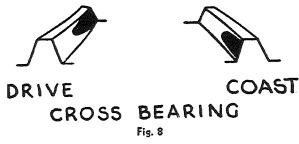
Fig. 8 shows a cross bearing. The gears are serviceable if the toe bearing is on the drive side and extends 5% the length of the tooth.
