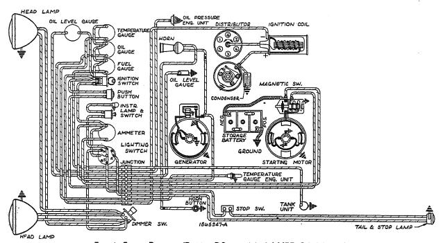
Fig. 4, Circuit Diagram (D-300, DS-300, Model HEF Cab-Murray)
