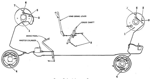
Fig. 1, Brake Adjustment Diagram
