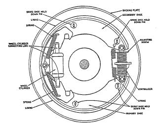
Fig. 3, Front Brake
