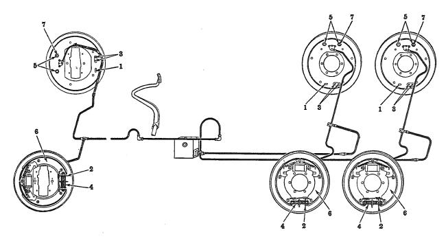
Fig. 1, Brake Adjustment Diagram
