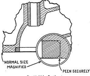
Fig. 16, Valve Seat Insert
