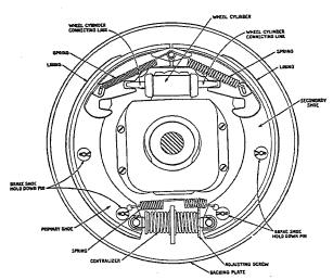
Fig. 4, Front Brake
