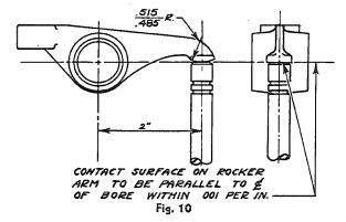
Fig. 10 illustrates the correct contact between valve and rockerarm end. The radius on rockerarm end must be held and under no circumstances should the end be ground off more than .010". The relation of the rockerarm end to the rockerarm bushing is also shown.
