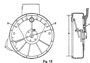
Engine must be supported before removing these parts.
