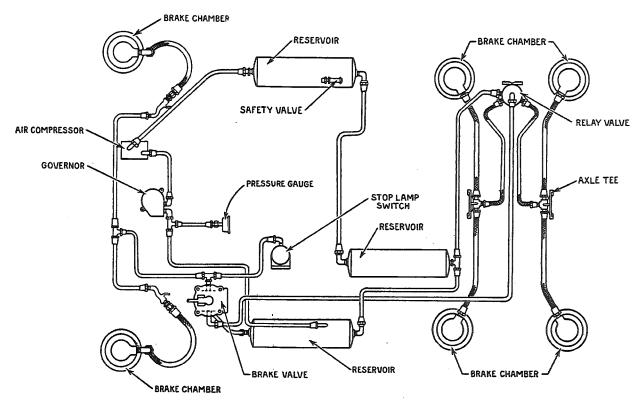
Fig. 1, Air Brake Installation Diagram
