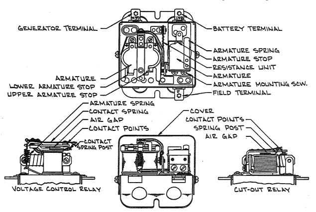
Fig. 3 (DR-5542) Step-Voltage Control Unit
