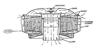
Fig. 1, Air Cleaner (D-2, D-15, D-30, DS-30, D-30B, DS-30B, D-186T, DS-186T)
