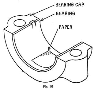
When assembling new connecting-rod bearings always start out with the specified quantity of shims in place. Then if bearing is loose, remove
