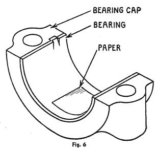
Connecting-rod bearing shims are assembled on side opposite tongue and groove side and is only side on which shims are used. Four .003" shims (two .006"-laminated-later models), are used (one side only) and if bearing wear cannot be adjusted to specified clearances by removal of shims, new bearing must be installed. Never file connecting rod or cap.
