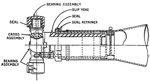
Fig. 1, 36 Splines on Slip Yoke
