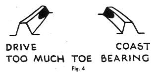
Fig. 4 shows too much toe bearing; gear must be moved away from pinion to increase length of bearing. A slight adjustment of pinion may be required to obtain proper profile bearing.
