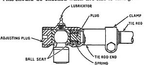
Fig. 2, Tie Rod Assembly
