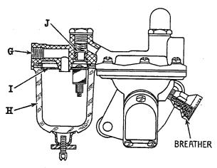
Fig. 3, Fuel Pump (FAB Series Engines)
