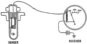
Fig. 5, Water Temperature Gauge—Cold
