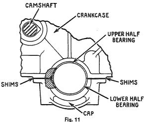
IMPORTANT: Before installing new bearings be sure to clean out drilled oil passages in crankshaft and block. A rifle barrel brush or a brass rod should be run thru the oil passages to dislodge any sludge, grit or bearing material. Plugged oil passages will prevent adequate lubrication to the new bearings, resulting in early failure.
