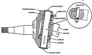
Fig. 1, Steering Knuckle Assembly
