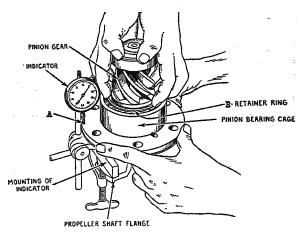
Fig. 12, Checking End Play of Pinion Bearing
