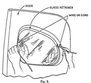
(f) Fig. 5 shows the progress of the retainer going into place. The upper left hand corner should go into place next, following with the upper right hand corner. Then work the lower right hand corner into place ahead of the lower left hand corner which should be the last corner to go into place.
