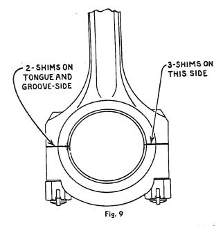
Connecting-rod bearing shims are assembled as shown in Fig. 9; three .003" shims opposite tongue and groove side and two .003" shims on tongue and groove side. If bearing wear cannot be adjusted to specified clearances by removal of shims, new bearing must be installed. Never file connecting rod or cap.
