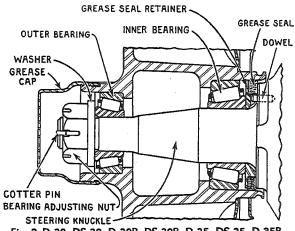
Fig. 3, D-30, DS-30, D-30B, DS-30B, D-35, DS-35, D-35B, D-40, D-186T, DS-186T, D-216T Front
