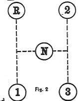
Move control lever to left and pull back to position (1).
