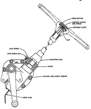
Fig. 1, R-720 Steering Gear
