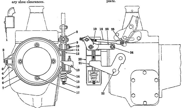
Fig. 2, Hand Brake (D-30, DS-30, D-30B, DS-30B, D-35, DS-35)
