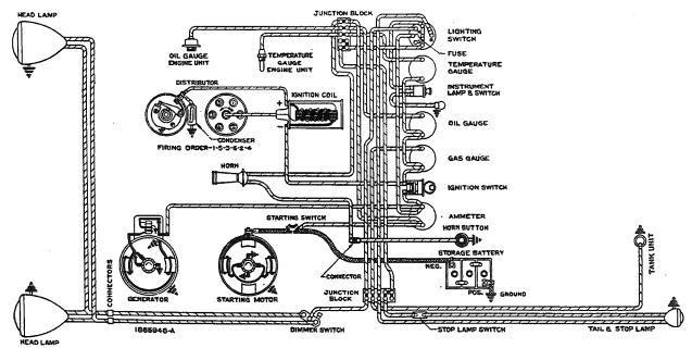
Fig. 1, Circuit Diagram (D-2, D-15, D-30, D-30B, DS-30, DS-30B, D-186T, DS-186T)
