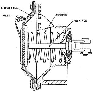
Fig. 6, Typical Brake Chamber (Diaphragm Type)
