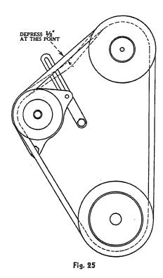
Belts should run under proper tension. Adjustment is made by loosening generator mounting screws and generator brace capscrew, after which generator can be moved in or out as required.
