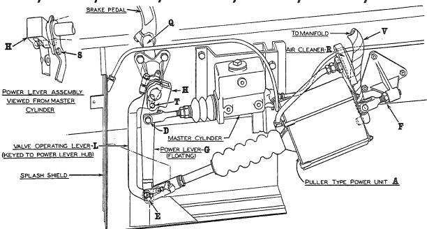
Fig. 1, Vacuum Power Unit Installation—D-35, DS-35, D-35B, D-40, D-50, D-60, D-186T, DS-186T, D-216T (See Page 4 for D-246T, D-246F)
