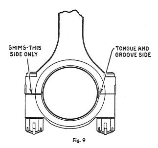
Connecting-rod bearing shims are assembled on side opposite tongue and groove side and is only side on which shims are used. Four .003" shims are used (one side only) and if bearing wear cannot be adjusted to specified clearances by removal of shims, new bearing must be installed. Never file connecting rod or cap.
