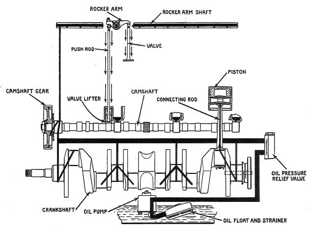
Fig. 27, Engine Lubrication System
