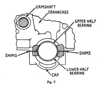
Two shims each .003" thick, are used on each side of main bearing, making a total shim thickness of .006".
