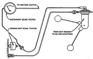
Two ten-foot lengths of insulated wire equipped with clip terminals at each end. These long lengths will in practically all instances permit individual making check to sit in seat of truck and observe gauge being checked.
