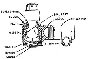
Fig. 3, Tie Rod Assembly—F-400, F-450, F-500, F-600, F-700, F-800 Axle
