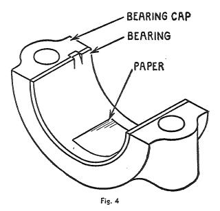
When assembling new connecting-rod bearings always start out with the specified quantity of shims in place. Then if bearing is loose, remove shims as required. Never build up clearance by adding shims, but reduce clearance by removing
