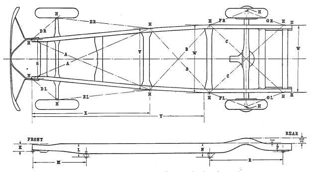
Fig. 1, D-2, D-5, D-15 Alignment Diagram (See Specifications)
