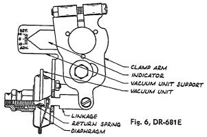
is opened slowly the vacuum is high and spark will be given additional advance to that of the centrifugal advance. On full load wide-open throttle when the vacuum is low or at high speed, the vacuum unit will not advance the spark. Under these low vacuum conditions spark advance depends upon the centrifugal mechanism in the distributor.
