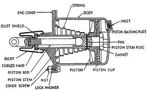
Fig. 7, Typical Brake Chamber (Piston Type)
