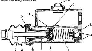
Fig. 1, Typical Combination Type Master Cylinder
