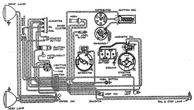
Fig. 3, Circuit Diagram (D-300, DS-300, Model HDM Cab-Burkett)
