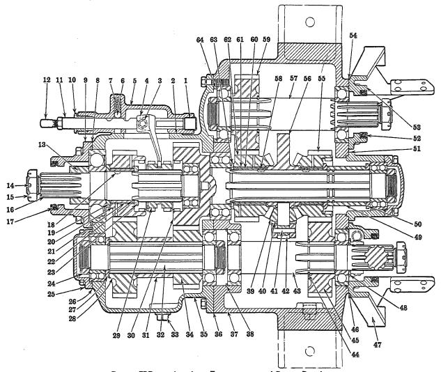
Fig. 1, FPD-45 Auxiliary Transmission and Power Divider
