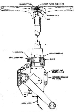
Fig. 1, R-320 Steering Gear
