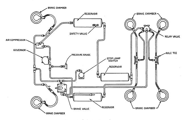
Fig. 1, Air Brake Installation Diagram
