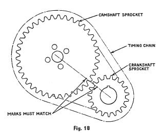
The sprockets are marked and should be installed so that the marks on camshaft and crankshaft sprockets match. Engine timing diagram is shown in Fig. 19.
