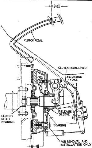
Fig. 5, Clutch Control (D-2, D-5, D-15)
