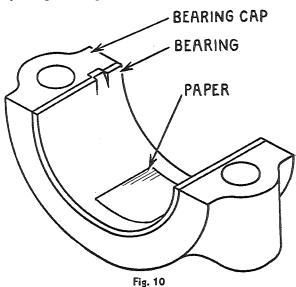
When installing new connecting-rod bearings always start out with the specified quantity of shims in place. Then if bearing is loose, remove shims as required. Never build up clearance by adding shims but reduce clearance by removing shims. This will prevent damaging bearing shells, by crushing, due to insufficient clearance.
