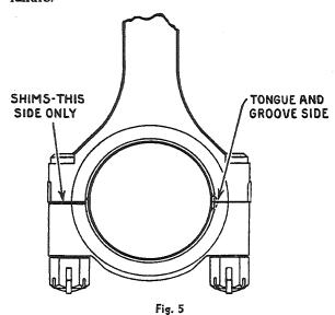
When replacing connecting-rod bearings be sure that rods and caps as well as backs of bearing shells are clean and smooth and free from oil. This is of extreme importance as bearings will not seat properly if there is any dirt or oil between bearing shells and rods or caps. Wash rods and caps in a good cleaning solution and dry thoroughly. This will remove oil as well as any dirt and insure proper contact between backs of bearing shells and rods.
