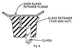
(b) Insert a piece of smooth insulated soft wire, or strong cord, approximately ½" diameter, around glass retainer groove which fits over metal flange of door glass opening. Cross the wire or cord on the top of the glass so the ends will be on the inside of the door. See Fig. 3.
