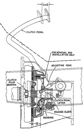
Fig. 6, Clutch Control (D-30, D-30B, DS-30, DS-30B, D-186, DS-186T)
