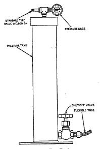
Fig. 37, Test Tank
