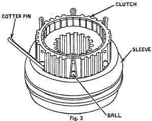
9. Disassembly of main shaft clutch assembly.
