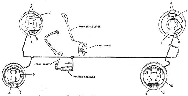
Fig. 1, Brake Adjustment Diagram
