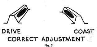
Fig. 3 shows the correct bearing on both drive and coast or reverse side of the tooth. The tooth bearing, both lengthwise and profile of the gear, should appear as shown. The profile bearing should fade out about ½2 to ½6" from top of gear tooth. Profile of the tooth bearing on the pinion will extend to the top of the tooth.
