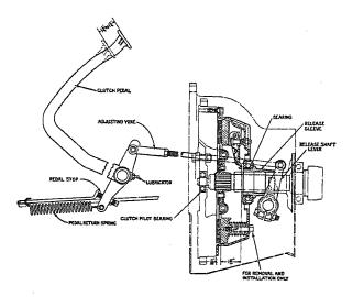
Fig. 10, Clutch Control (D-300, DS-300)
