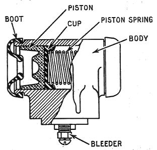
Fig. 3, Typical Wheel Cylinder
