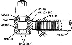
Fig. 2, Tie Rod Assembly—F-300, F-301\_Axle
