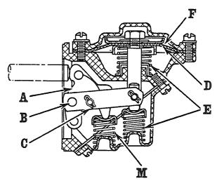
Fig. 2, Fuel Pump (FAB Series Engines)
