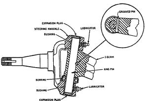
Fig. 1, Steering Knuckle Assembly
