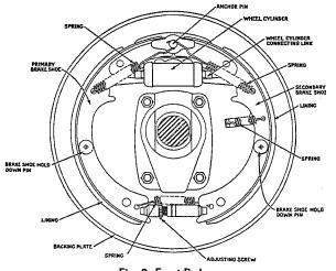
Fig. 2, Front Brake
