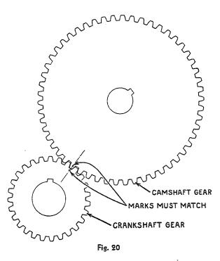
Timing gears must be installed so that the crankshaft and camshaft are in correct relation to each other. Gears are marked and should be installed so that marks on camshaft and crankshaft gears match. Engine timing diagram is shown in Figs. 21 and 22.
