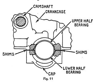
IMPORTANT: Before installing new bearings be sure to clean out drilled oil passages in crankshaft and block. A rifle barrel brush or a brass rod should be run thru the oil passages to dislodge any sludge, grit or bearing material. Plugged oil passages will prevent adequate lubrication to the new bearings, resulting in early failure.
