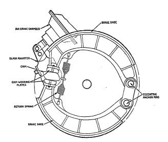
Fig. 2, Front Brake
