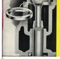
Left: Hardened exhaust-valve seat inserts retard valve-seat burning and retain engine efficiency.
