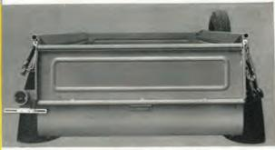
The two-piece, box-type, welded tailgate has concealed hinges and drops level with the floor, where it may be supported with rubber-covered side chains or dropped straight down. The embossing in the tailgate adds a distinctive note as does the skirt below the tailgate.
