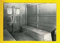
This view of the interior of the 25-case capacity, type DM milk body (DB body for bakery use) shows the sturdy, reinforced construction, and presents some idea of the large load area provided. Sufficient work space for the delivery man speeds up the service and helps to cut costs. All features of the body as well as the Models D-2 and D-5 chassis combine to provide a complete truck which meets the demands of utility and economy in door-to-door delivery.
