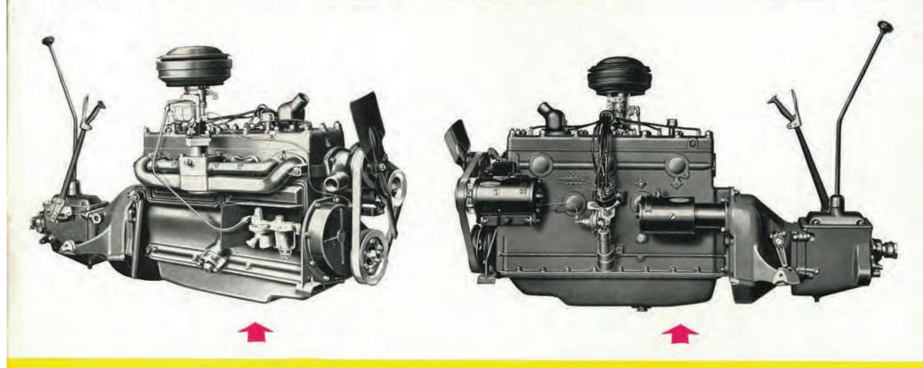
Right front view of the Model D-2 six-cylinder, L-head engine, clutch and transmission, showing the oil-bath type air cleaner, downdraft-type carburetor, fuel pump, manifold, and the newly designed fan. This engine develops 78 maximum brake horsepower at 3,400 r.p.m. and maximum torque of 155 lb.-ft. at 1,000 r.p.m. The D-2 "economy" engine develops 45.9 maximum brake horsepower at 3,000 r.p.m. and a maximum torque of 107 lb.-ft. at 800 r.p.m.
