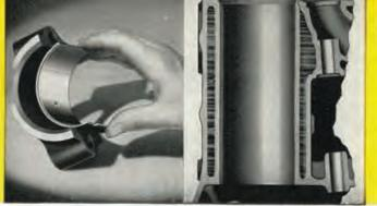
Left: Water jackets, extending the full length of the cylinders in the Model D-2 engines, assure positive cooling.
