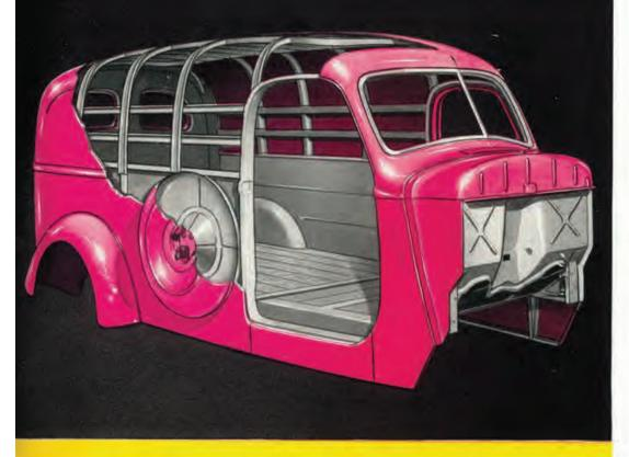
These strong, safe, welded-steel de luxe panel bodies are fabricated like a skyscraper. Cutaway view shows the rigid construction of the unit, how the side pillars are welded to the roof assembly, the longitudinal steel channel ribs, the pressed-in tire carrier pocket, the cowl and dash assembly, and other construction details.
